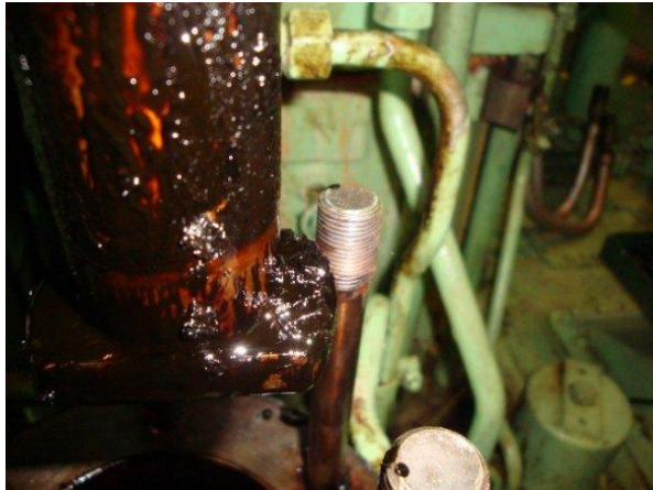
Stuck fuel pumps with sludge
