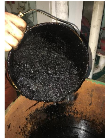
Sludge in fuel tanks
