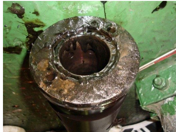
Stuck fuel pumps with sludge
