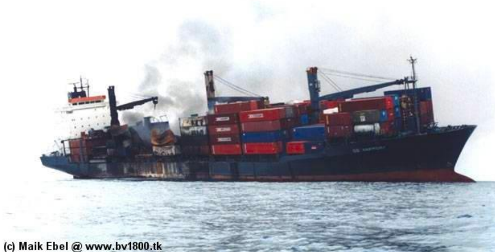
Figure 7: "DG HARMONY" burning after the explosion of calcium hypochlorite [Source: Maik Ebel, www.bv1800.tk]
