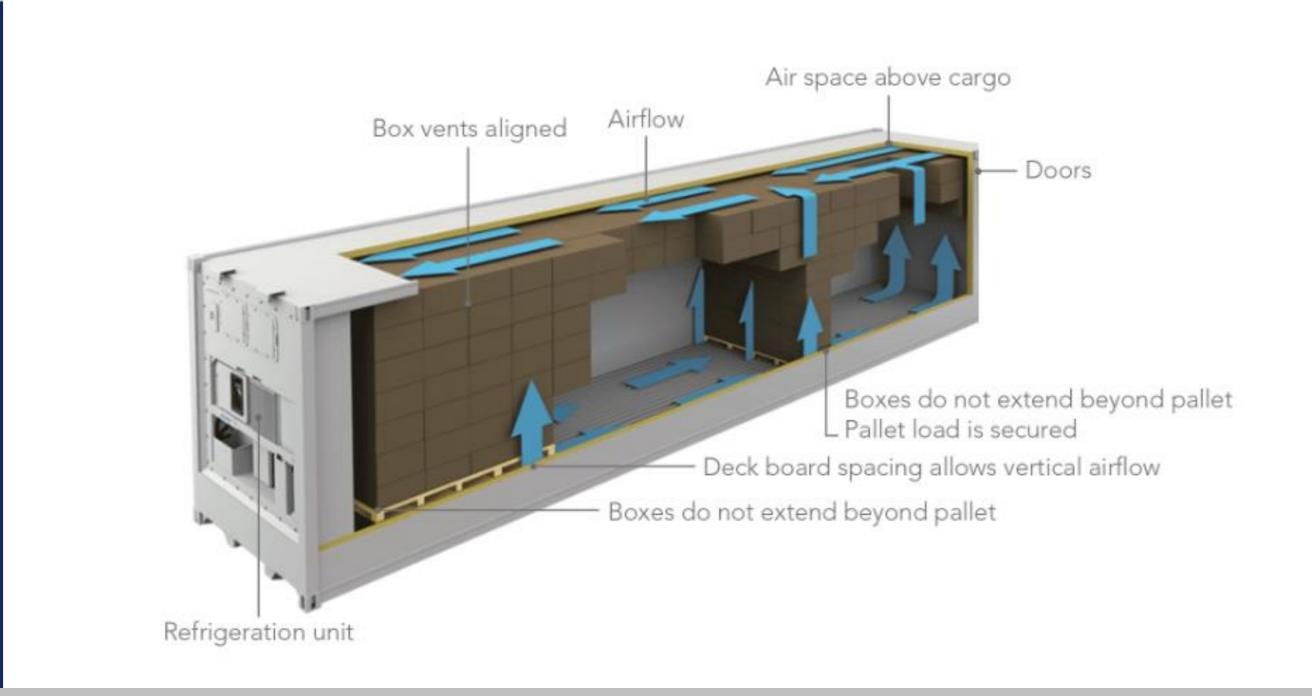
Airflow: from bottom (from cold compartment through the T floor surrounding and in vertical ascension in the load and return by the top)
