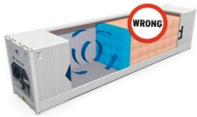
Air short circuit and/or air flow reduction/blockage
