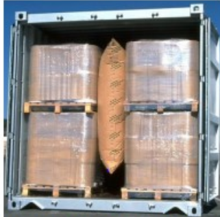
Figure 7.9 Gap filled with a central dunnage bag
