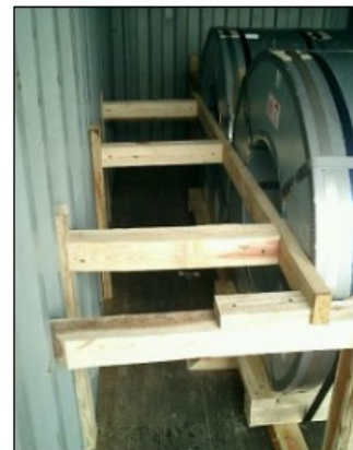
Figure 19: Improper transfer of pressure to the container walls and poor stabilising of shores
