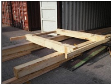
Figure 3: Timber structure for bedding a cable drum in front of a container
