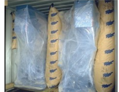
Figure 7.10 Irregular shaped packages blocked with dunnage bags
