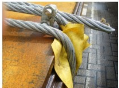
Figure 7.11 Poor edge protection
