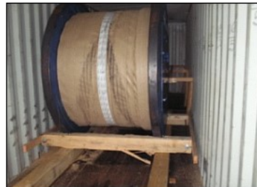
Figure 4: Cable drum on its bedding in the container
