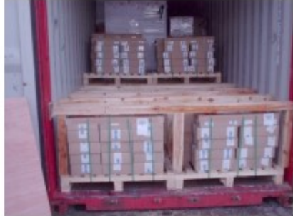
Figure 7.2 Timber temporary floor
